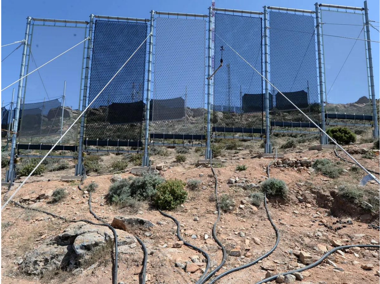
A photo illustrating the fog harvesting technique in a remote village in Morocco. Source: Alarabiya.net
